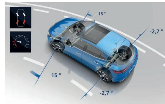
At speeds below 60km/h (below 80km/h in Sport mode), the rear wheels turn 2.7° in the opposite direction of the front wheels.
